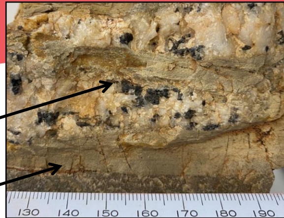
Cassiterite from Tallebung – Scale in mm
