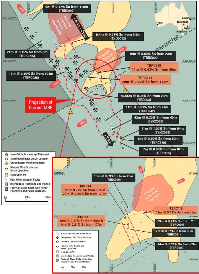
*Figure 1:* Plan showing the current boundary of the Tallebung MRE with new intercepts shown in orange. Past highlight intercepts are shown in black. Inset shows southern open pit area with new results.
