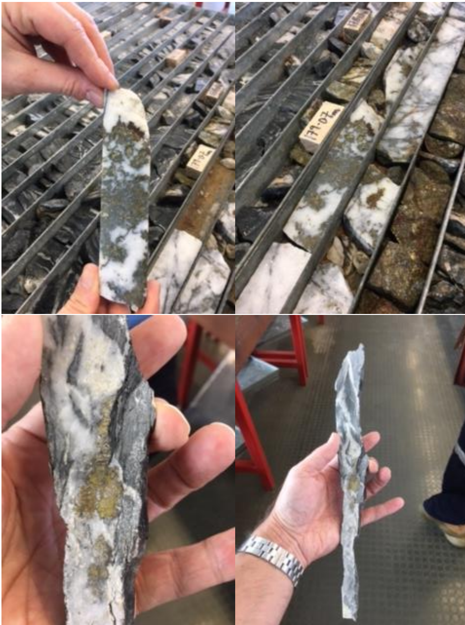
Above: strong veining and sulphides in Iron Duke core not previously sampled
