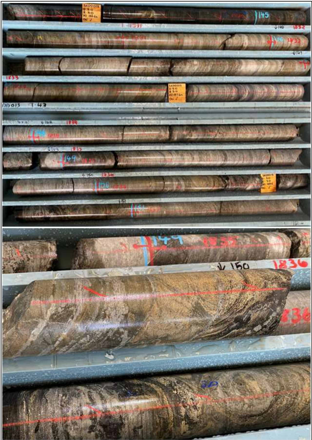
Figure 1: 3KEL Target – Top: Diamond drill core in trays from first hole 3KDD013, 144.1-151.6m DH. Bottom: Close up of drill core from 150.3-150.4 with pale honeycomb coloured semi-massive sphalerite – Assays are pending.
